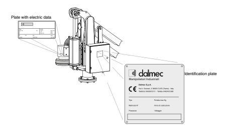
The electric specifications of a possible vacuum generator are indicated on a plate placed on the generator itself.
